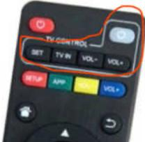
2. Press the key to learn (such as power), the red-light flashes, and the remote control is in the learning and receiving state.
