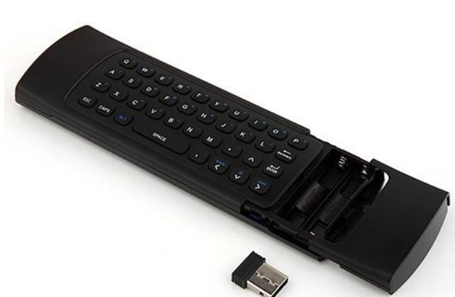
Insert the batteries and press any button/key on the remote to test whether the batteries are inserted correctly. This will be confirmed by the red LED lighting up every time you press a button of the remote. If this is not the case, then check the batteries if correctly inserted or replace them.
